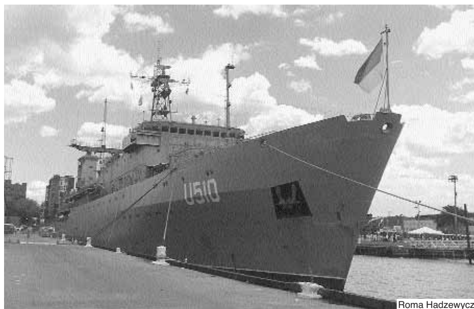
The Slavutych, 106 meters in length, with a beam of 16 meters and a displacement of more than 5,000 metric tons.
